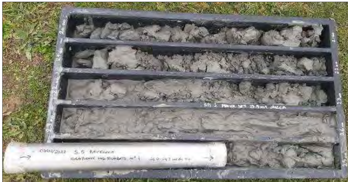
Figura 39. Sondaggio S5 cassetta 20,0-25,0 m
