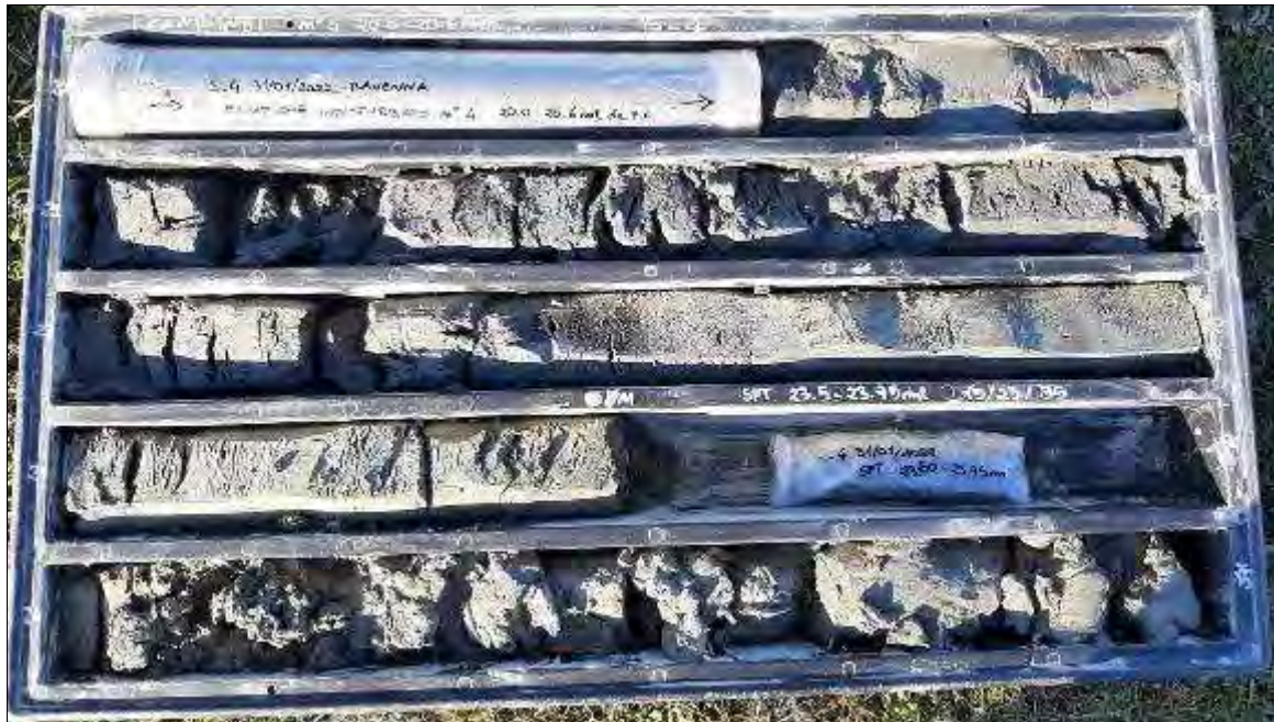
Figura 31. Sondaggio S4 cassetta 20,0-25,0 m
