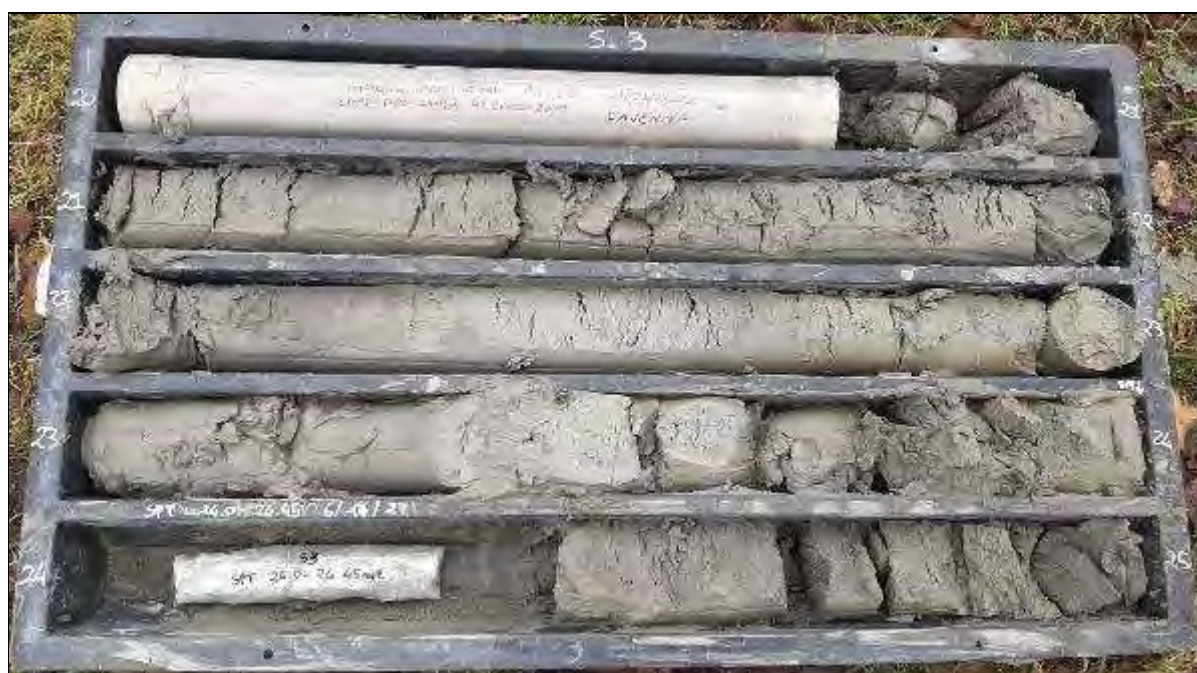
Figura 22. Sondaggio S3 cassetta 20,0-25,0 m
